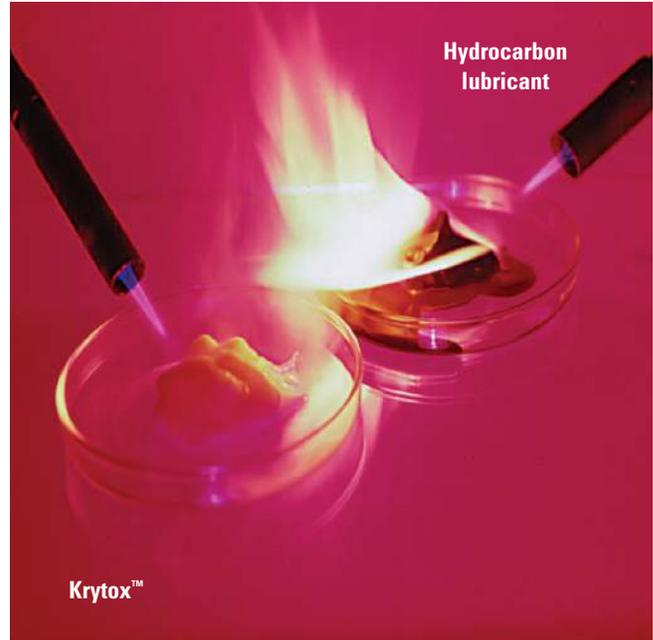
Hydrocarbon-based lubricants burn; Krytox™ lubricants do not.
